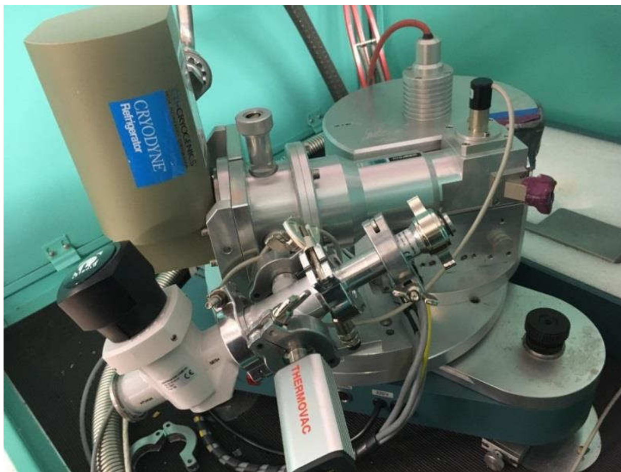
Figure 14: Photo of chamber and cooling system of cryostat
