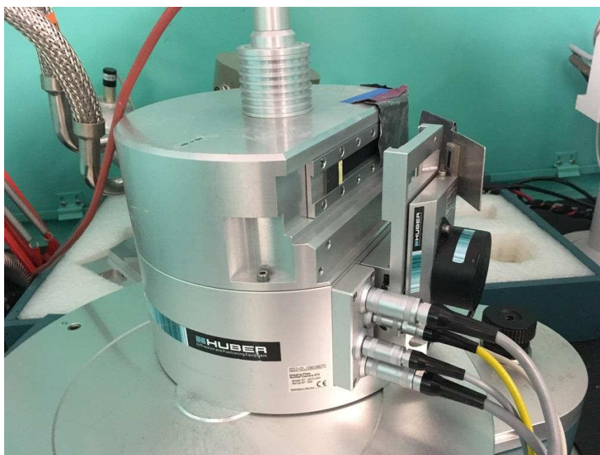
Figure 13: Photo of Image plate detector system of the Huber diffractometer with housing
