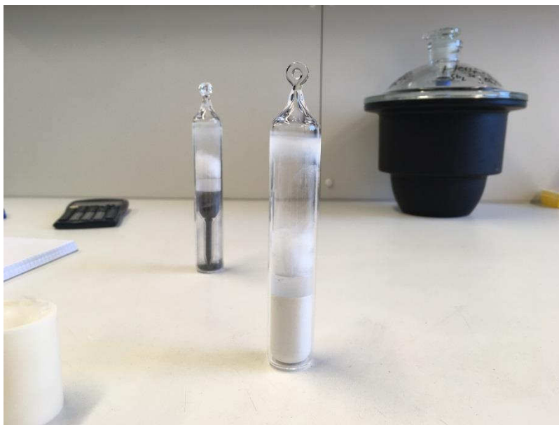
Figure 16: Synthesis variant A. The tubes contain the sample before the melting process.
