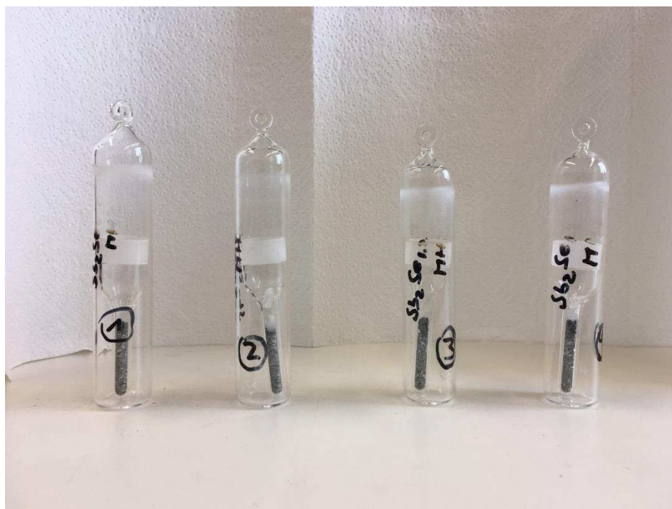
Figure 17: Synthesis variant B and C. Tubes contain the sample before the melting process.
