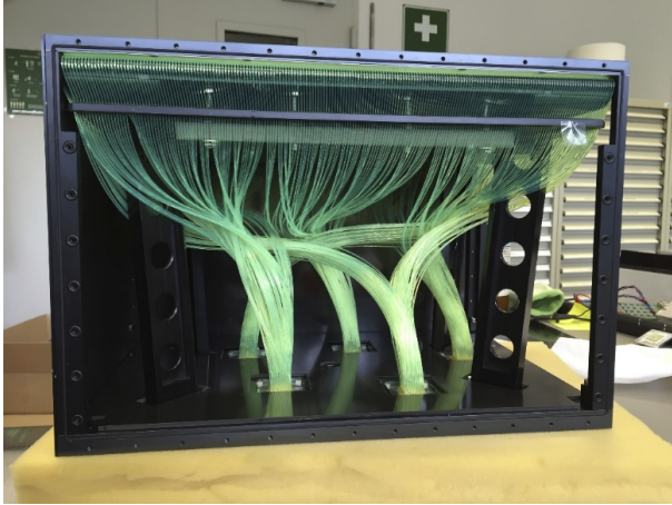
Fig. 2.8: Fiber guidance in the detector. On the top there is the orthogonal WLSF array sandwiched by scintillator screens (not visible). The fibers are bent backwards and merged into five bundles, and a MaPMT is mounted behind each bundle. Note that opposite ends of each fiber are fed into the same MaPMT pixel.
