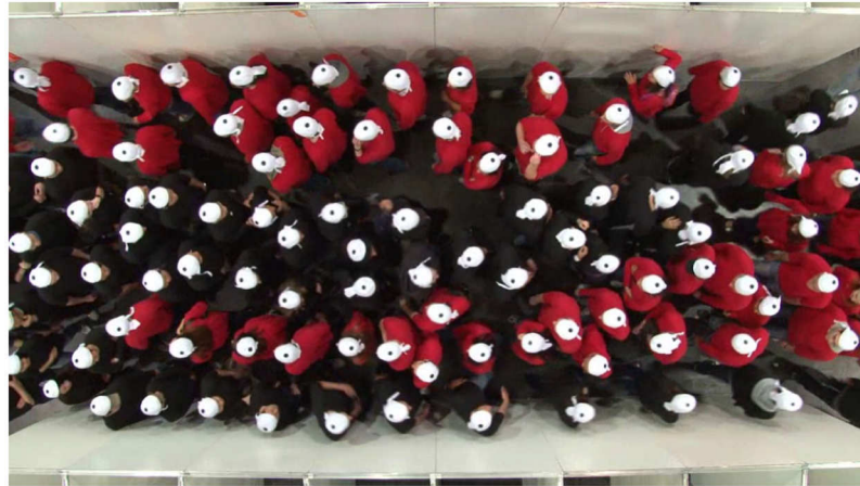
Fig 1. Snapshot of an experiment with bidirectional pedestrian streams. Test persons with black shirts are moving from left to right (red shirts from right to left). Lanes unstable in time and space are formed. For a movie of this experiment we refer to supporting information S1 Movie .
