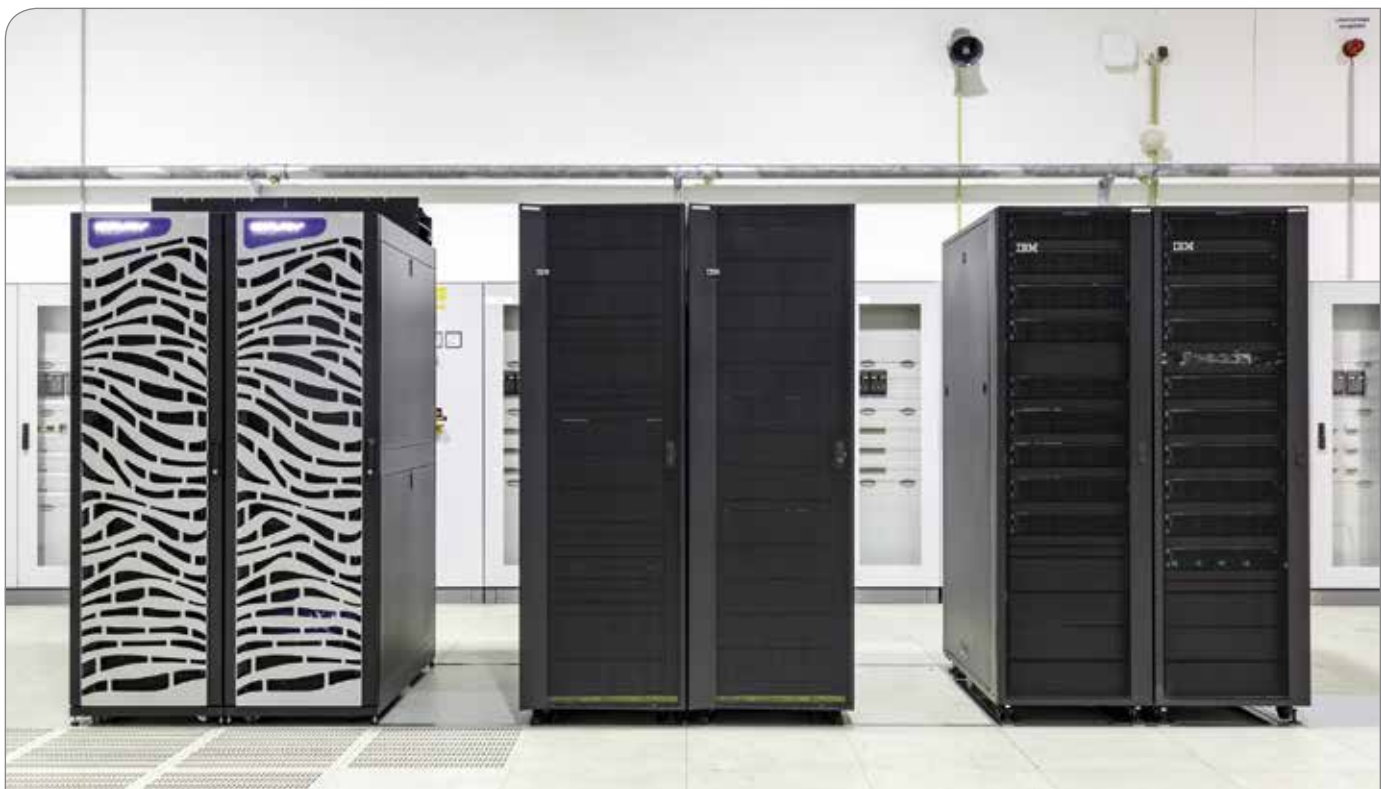
The two pilot systems, developed by Cray (left) and IBM-NVIDIA (right), are designed to meet the specific requirements of neuroscience applications. Both systems are connected to an high-performance storage system from IBM/Lenovo (middle).
