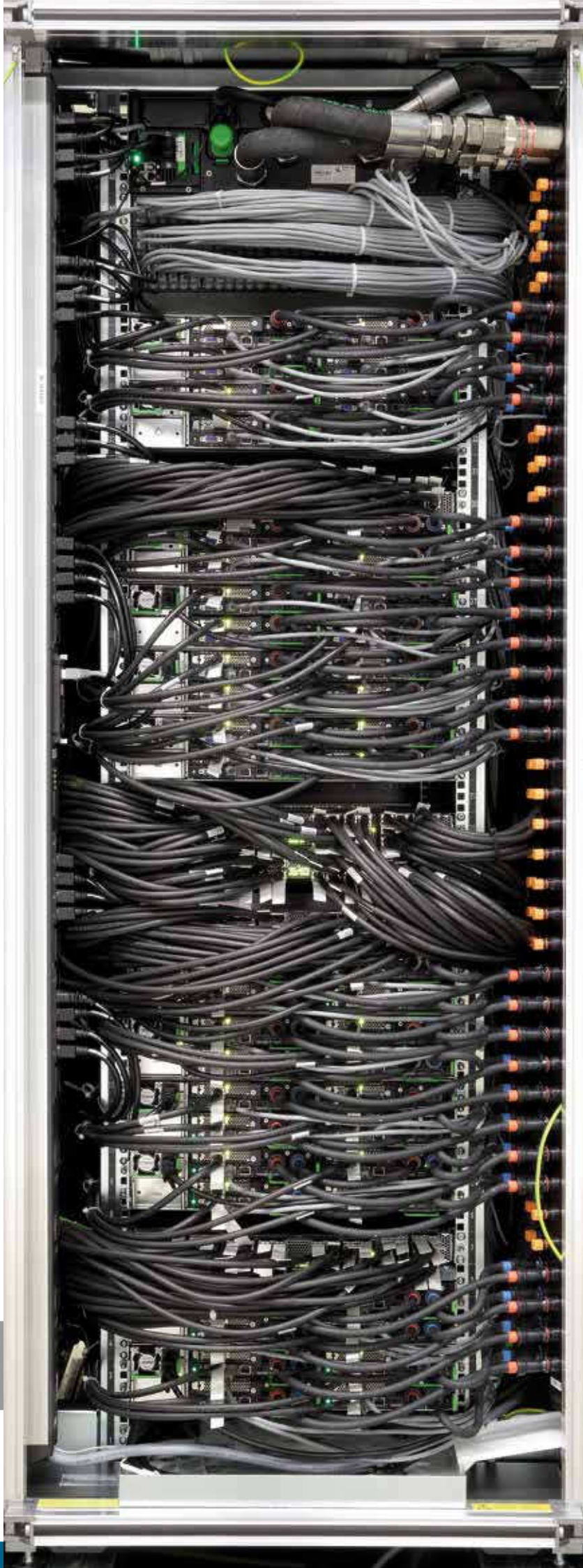
Single QPACE 3 rack with a water manifold at the right side, which is connected to a heat exchanger in the top of the rack.
