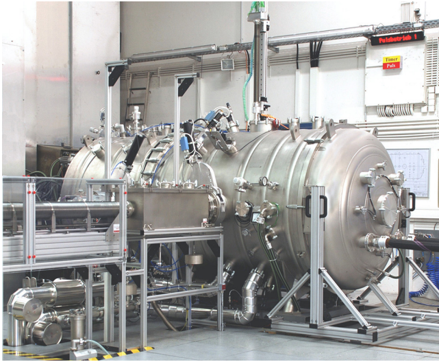
Figure 5. GLADIS neutral beam facility. The vacuum lock for target exchange is visible in front of the vessel.
