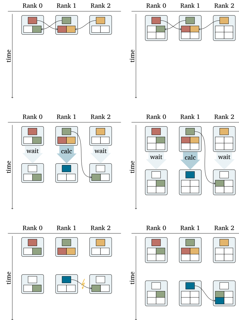
Figure 6.1: Single buffered method (left) compared to double buffered method (right). Within one dimension three ranks are communicating with each other (thin arrows). The big rectangles with rounded corners represent the memory of each rank, while the smaller rectangles inside represent the communication buffer. The single upper rectangle stands for the sending buffer, while the lower rectangles represent receiving buffers. White filled rectangles denote empty buffers, whereas colored rectangles represent buffers with valid data.
