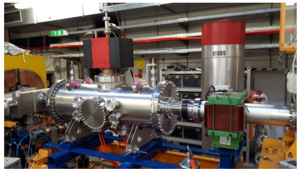
Figure 4: First HESR kicker installed at COSY.
