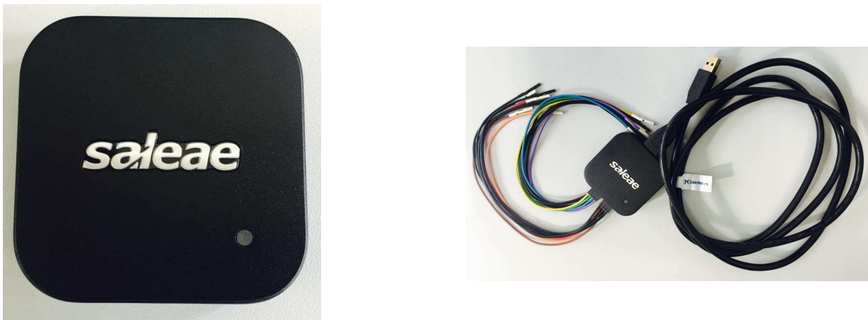
Figure 3.7: Saleae Logic Pro 8 Analyzer
