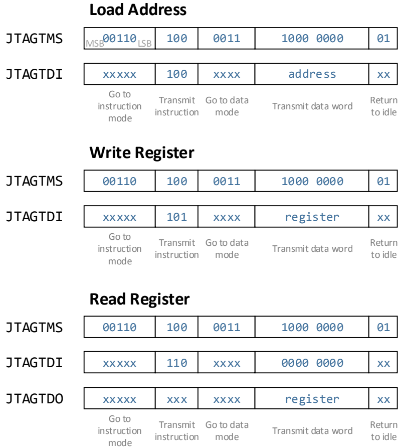
Figure 2.8: Exemplary sequences for register interaction, an x represents an undefined state. Transmission in each block is starting from the LSB to MSB
