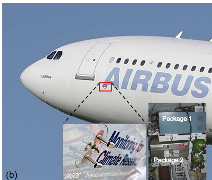
Figure 1: a) Schematic scheme of the temperature sensor attached to the humidity sensor mounted in the Rosemount housing (Helten, 1998). b) Packages 1 and 2 installed aboard the AIRBUS A340-300, and the inlet plate including the Rosemount housing (photograph by courtesy of Lufthansa).
