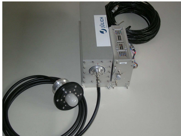
Figure 1. Basic components of a CCD array spectroradiometer system for airborne measurements. The 2\pi receiver optics with optical fiber (black, front), spectrometer including the monochromator and CCD array detector (middle), and the cooling electronics (right).
