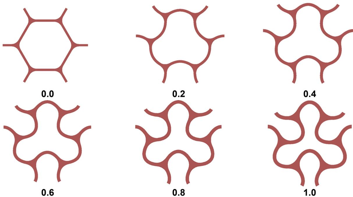
**Fig. 2.** Modeled evolution of a honeycomb cell with increasing lithium concentration, indicated by the numbers.
