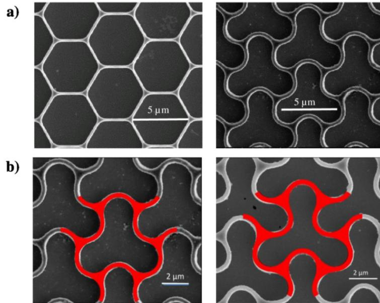
**Fig. 1.** a) Morphology of honeycomb-structured Si anode before lithiation (left) and after lithiation (right) observed in experiments [9]; b) overlay of experimental and simulated (red) cell patterns: lithium loading of 45 % (left) and 80 % (right).
