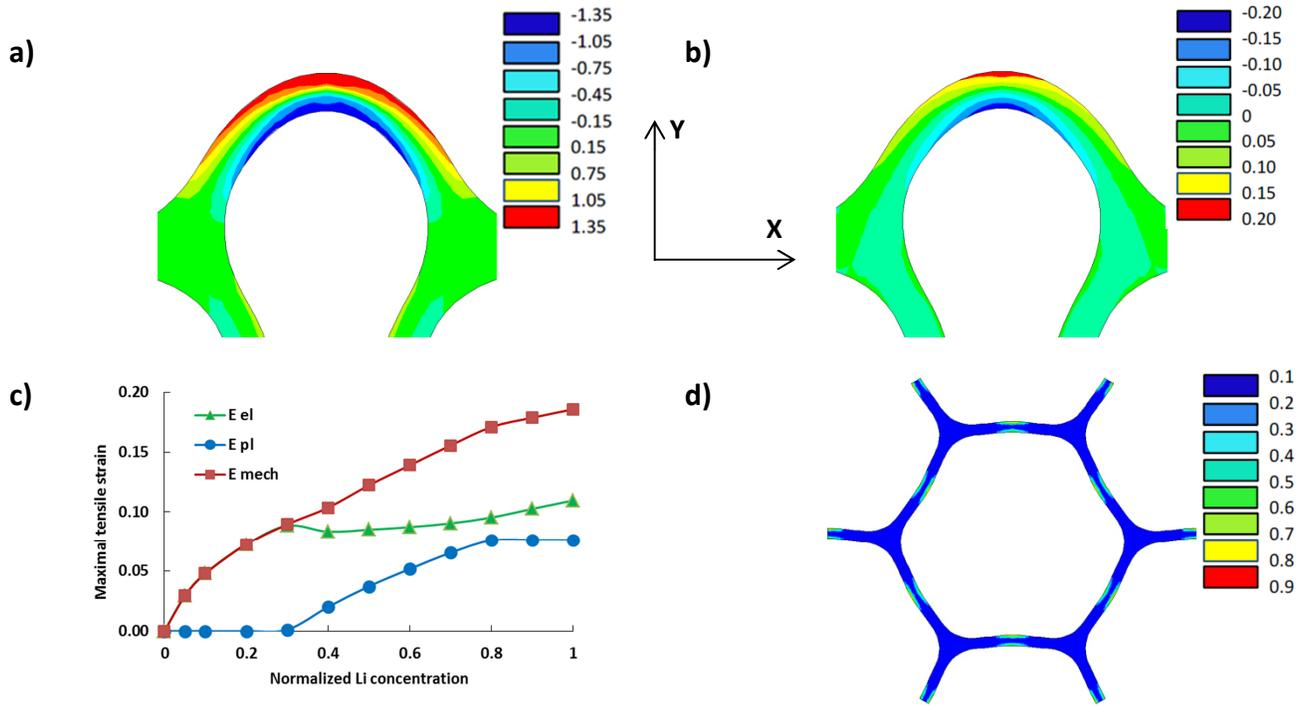
**Fig. 3.** a-b) Distribution of equivalent stress (a) and equivalent strain (b) across the wall of a fully-lithiated honeycomb; c) Modeled variation of the maximal elastic ( $E_{el}$ ) and plastic ( $E_{pl}$ ) strains, and their sum ( $E_{mech}$ ) in the honeycombs with increasing lithium concentration; d) Modeled honeycomb cell after full lithiation and subsequent full delithiation. The contours show the residual maximal plastic tensile strain.
