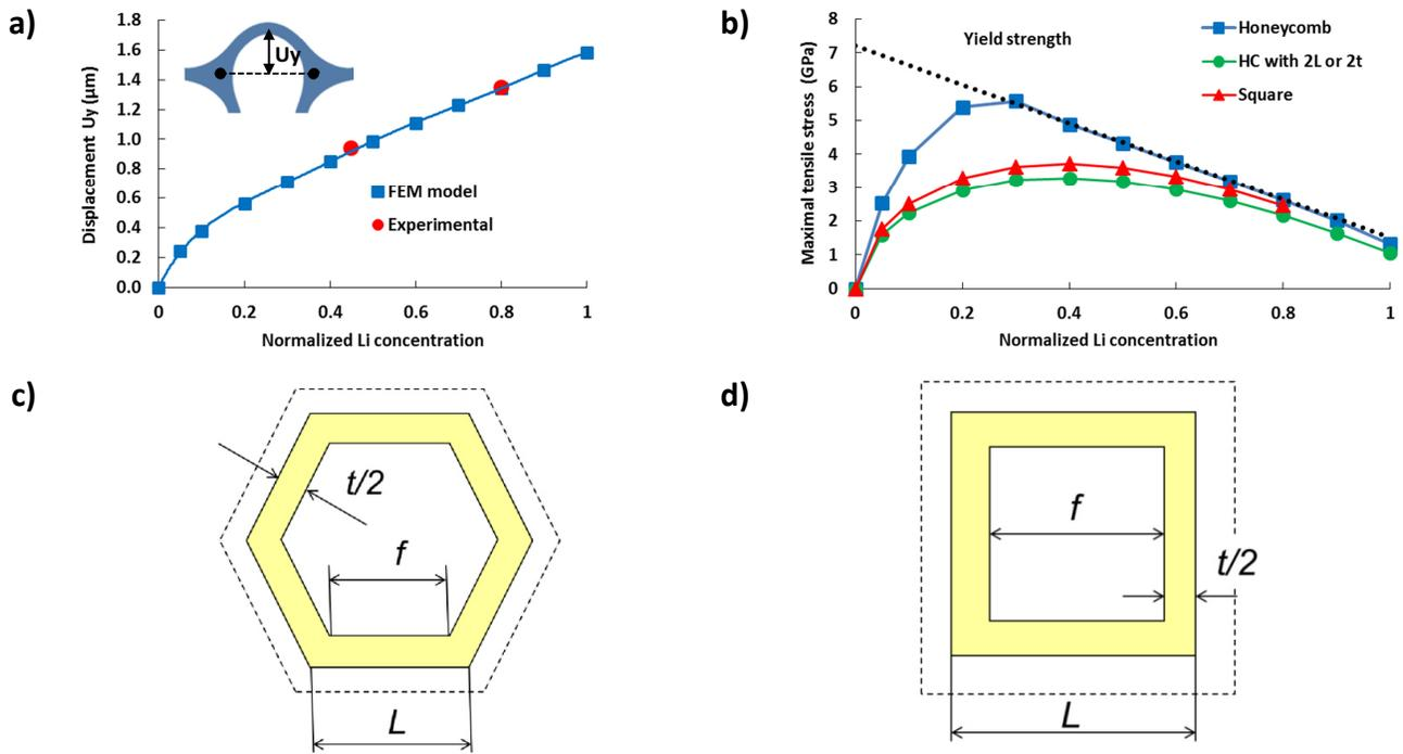
**Fig. 4.** a) Modeled and experimental displacement of middle point of the honeycomb (HC) wall vs. Li concentration; b) Evolution of maximal tensile stress during lithiation of Si with various cellular architectures; c-d) Schematic representation of single cell geometries used to calculate the storage capacity per unit footprint area: c) Honeycomb-based microstructure; d) Square-based microstructure.
