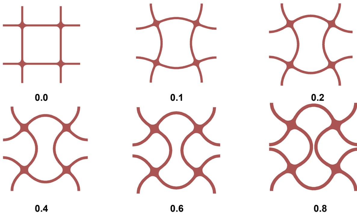
**Fig. 5.** Modeled evolution of a square Si-cell with increasing lithium content, indicated by the numbers.
