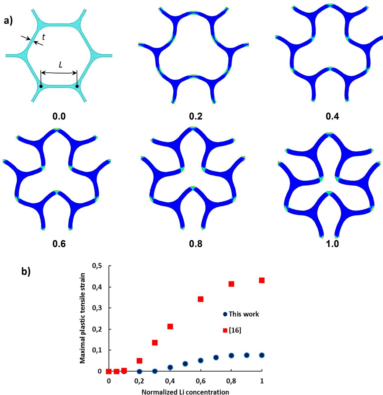
**Fig. S1.** a) Modeled evolution of a honeycomb cell with increasing lithium concentration (indicated by the numbers) with a yield strength of 3.6 GPa for pristine Si and 0.7 GPa for fully lithiated Si [16]. The contours show the maximal plastic strain penetrating the honeycomb wall; b) Maximal plastic strain evolution modeled with the yield strength used in this work and with that reported for Si nanowires [16].
