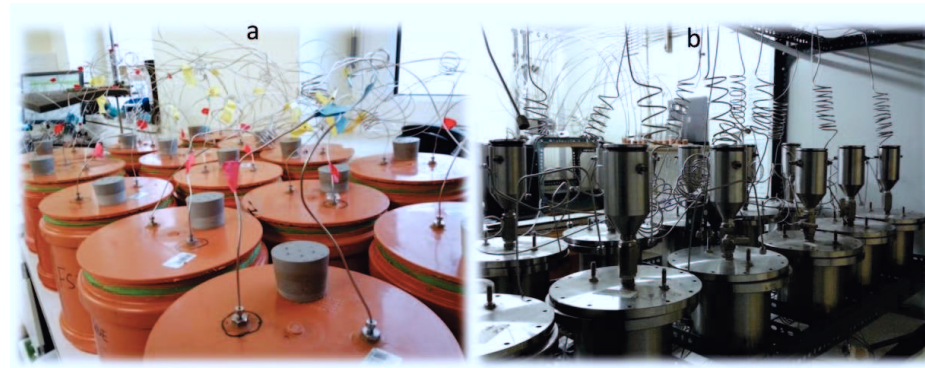
Figure 3. The two automatic incubation systems (a) used in Paper II and V and (b) used in Paper I and III.
