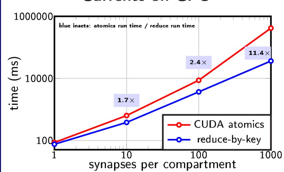
Time taken to update 10'000 compartments as the number of synapses per compartment varies. Race conditions occur when multiple synapses on the same compartment update compartment current simultaneously. Arbor has an optimized reduce-by-key operation that improves performance over naive CUDA atomics when many synapses are attached to the same compartment.
