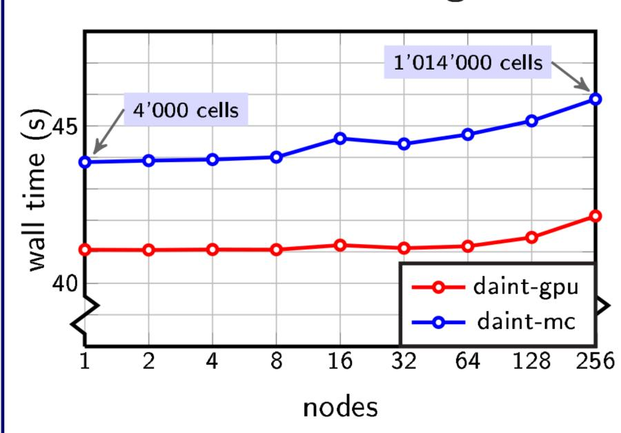
Time to solution with 4000 cells per node, as the number of nodes is increased. Run time increases by less than 25% when the problem is scaled by  $256 \times$ . Arbor has a dry-run mode that was used to tune scaling issues with many nodes.
