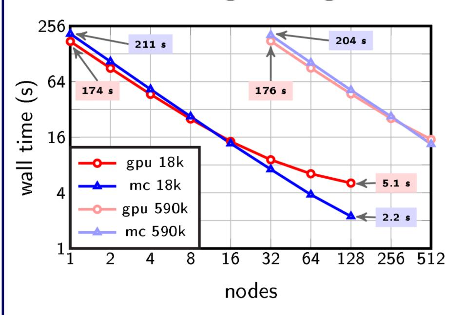
Time to solution on CPU and GPU for models with 18'000 and 590'000 cells. GPU performance is better in "throughput mode", i.e. with more cells per node, while CPU is faster with fewer cells per node.
