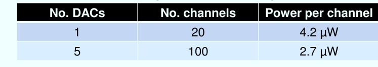
→ DAC architecture and global signals promise further reduction of power consumption
