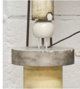
Figure 4-5: Compressive creep test set-up.
