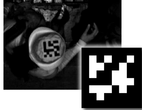
Figure 2. Top left: person wearing a hat with a Reed-Solomon code marker used in the experiments of the project BaSiGo. Bottom right: example of the ARUCO code marker consisting of a solid border for easier detection and an inner 6 \times 6 bit code.
