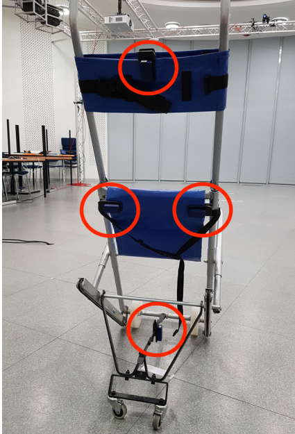
Fig. 2. Evacuation chair equipped with four IMUs marked with red circles.
