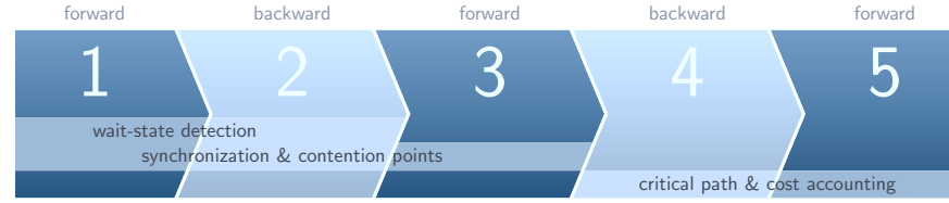
Figure 4.5.: Five consecutive replay phases used in Scalasca. Each phase can use data structures built up in prior phases. The replay direction is indicated by the heading and color of the individual phase. Wait states are detected in the first two phases. Contention point data is computed in the first phase, while synchronization point data is computed in phases one through three. Once synchronization and contention point data is computed, phases four and five assess the overall costs and the critical path.
