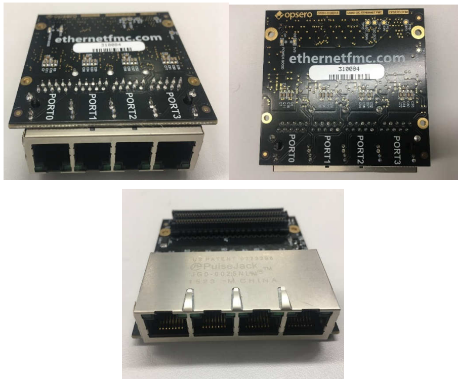
Figure 3.2 Ethernet FMC module or adapter for FPGA
