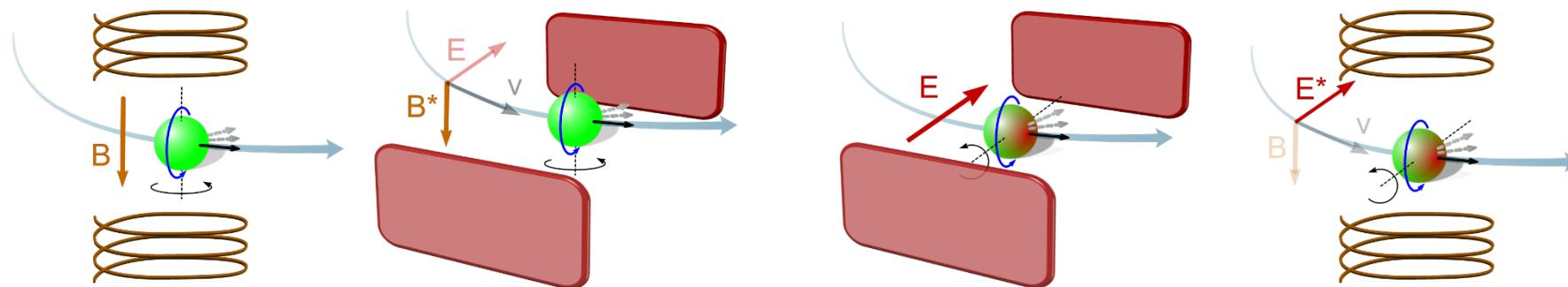
**Magnetic moment** causes fast spin precession in horizontal plane
