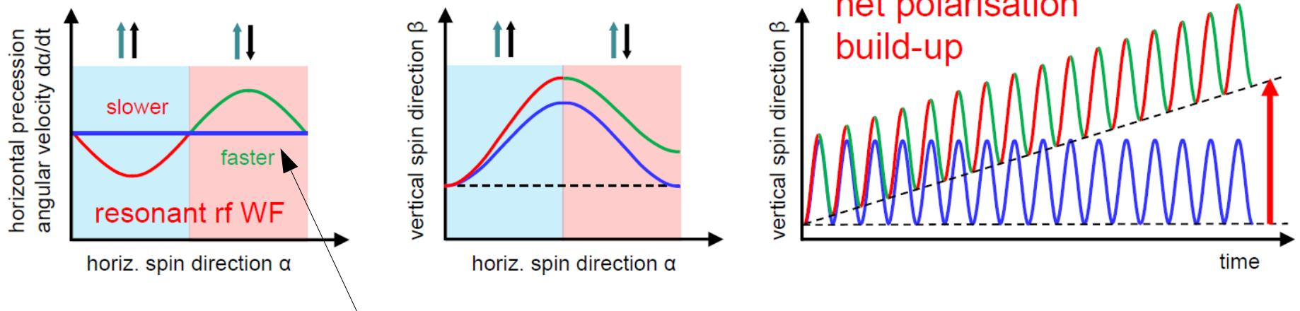
Wien Filter has to be always **in phase** with the horizontal spin precession!
