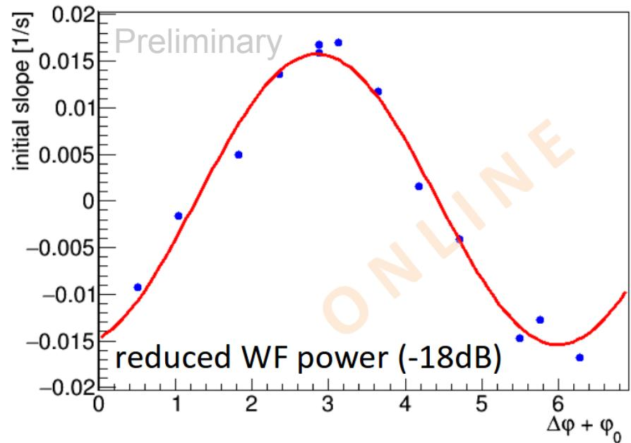
Spin build-up as a function of phase  $\sim \sin\Delta\varphi \rightarrow$  Feedback system works properly!
