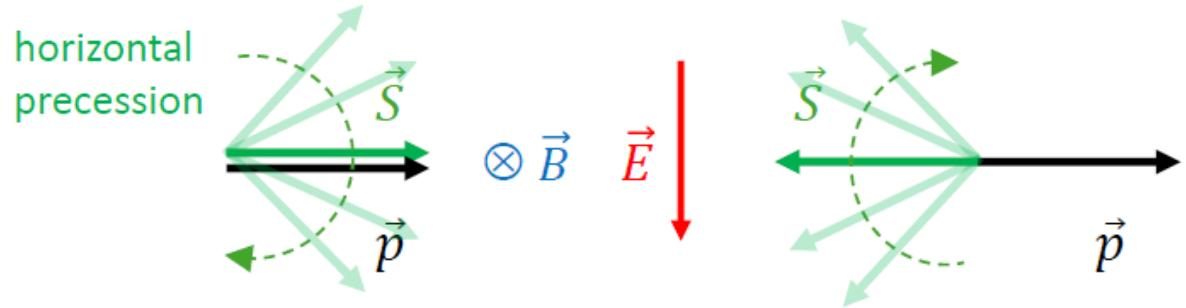
Wien Filter: introduces  $B$  and  $E$  field oscillating with radio frequency
