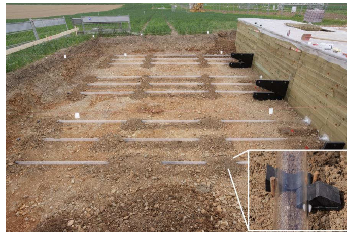
Fig. 2. 1 Installation of the minirhizotron facility in the upper part of the test site. The wood container is the accessible facility. Wedge-shaped fixture blocks shown in the right corner were used to fix the tubes during soil backfill.
