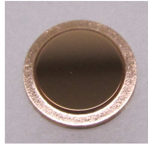
Fig. 2.9: Photograph of new Cu (111) single crystal with hat shape cut.
