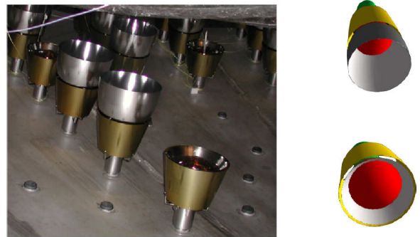
FIG. 6. Left Panel: Real Borexino inner detector PMTs mounted on the stainless steel sphere. Right Panel: MC schematization of the PMTs with (top) and without (bottom) light concentrators.
