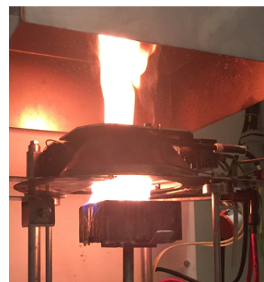
Figure 4: Cone Calorimeter experiment.
