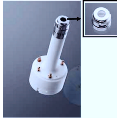
Figure 4.1: Design of the SPECS sample holder along with the mounted cap. Adapted from [40].
