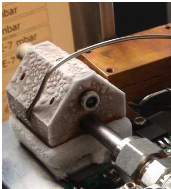
Figure B 2: Frost generated on the collector of the ACM during collection. Before changing to the desorption mode the collector was first heated up to 20 °C in order to disconnect the peltier element using the lifter.
