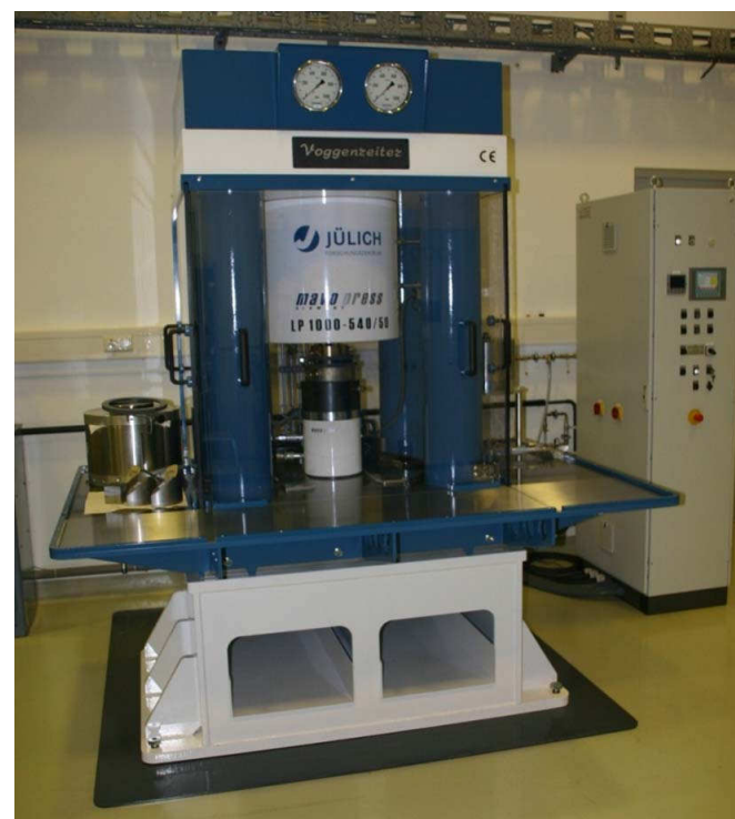
Fig. 14: Combined piston cylinder / multi anvil press. In this picture the piston cylinder module is installed under the main cylinder. On the left workbench side of the device the walker-type multi anvil module is visible.
