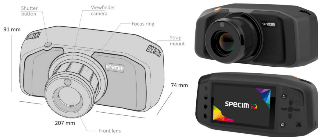
Figure 1. Vector visualization of the Specim IQ (Specim Ltd., Oulu, Finland) with annotations and dimensions on the left side and RGB renderings on the right side.
