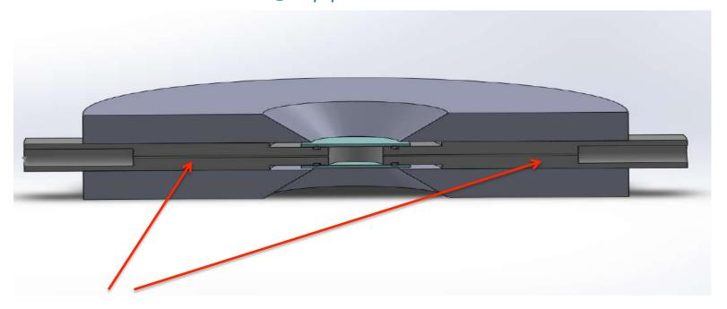
The exchange of the mother liquor is allowed by means of two capillarity built in the spacer
