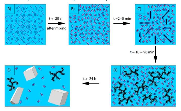
The crystal growth is due to not only by the addition of small dimers, but also of large fractal aggregates.
