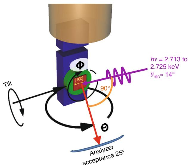
**Fig. 2** The experimental geometry with various key parameters shown. Azimuthal angle  $\Phi$ , polar and beam incidence angles  $\theta$ ,  $\theta_{\text{inc}}$ , and tilt angle are indicated. Light scattering plane runs along [100] crystallographic direction
