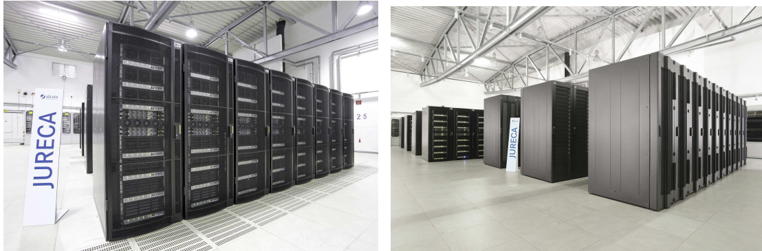
Figure 1: Jülich Research on Exascale Cluster Architectures (JURECA) at Jülich Supercomputing Centre. The left picture shows the Cluster module in 2015. The right picture shows the complete system after the Booster deployment in 2017. Copyright: Forschungszentrum Jülich.
