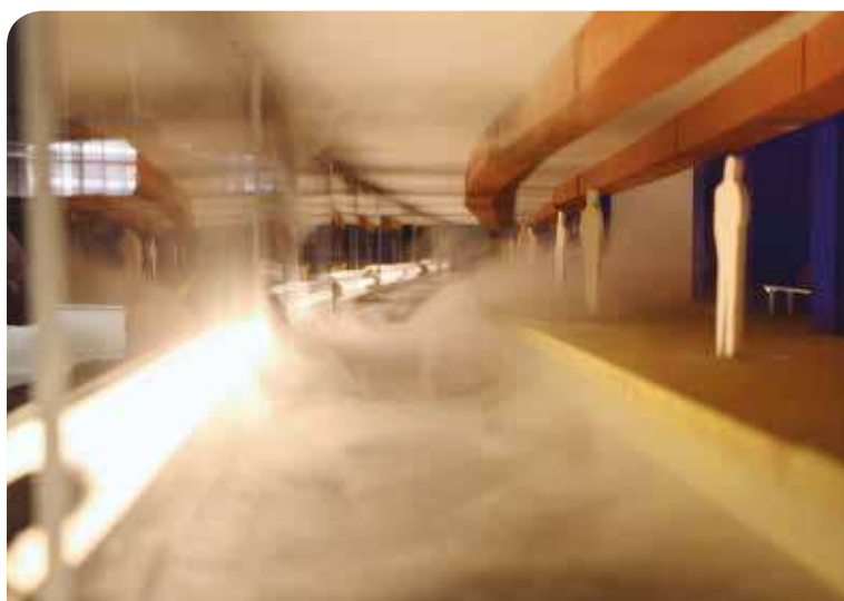
Fig. 3: Inside view of the 1:15 scaled model of the metro station 'Osloer Strasse'. Small-scale smoke sources are used to model the smoke spread. © Lukas Arnold
