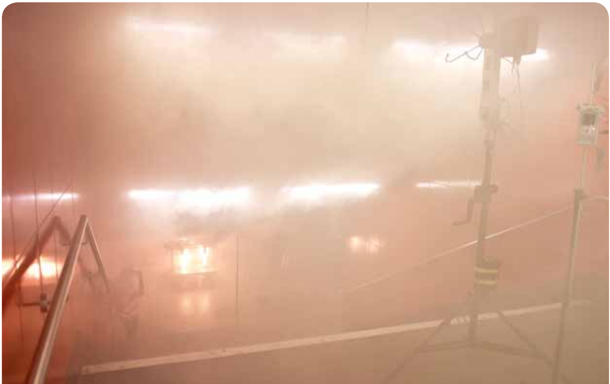
Fig. 1: Real-scale fire experiment in the metro station 'Osloer Strasse' in Berlin. Propane burners simulate the initial phase of a fire, while the full station is monitored with temperature and concentration sensors. © Lukas Arnold
