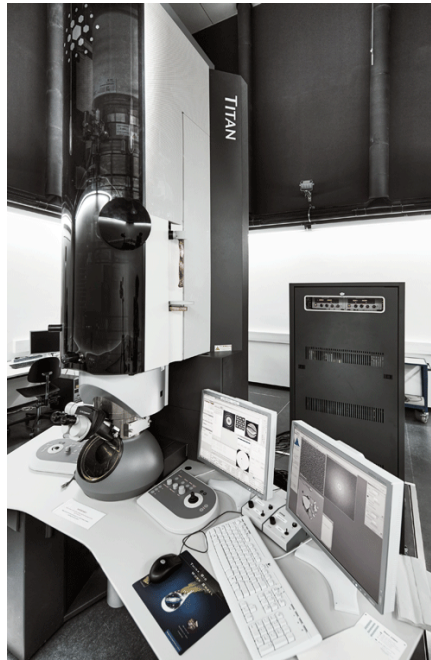
Figure 1.1.: Picture of the FEI Titan G2 60-300 HOLO, installed in the Ernst Ruska-Centre for Microscopy and Spectroscopy with Electrons (ER-C) in the Jülich research centre. This fourth generation TEM is optimised for the investigation of electromagnetic fields in materials using off-axis electron holography. Image taken from [44].
