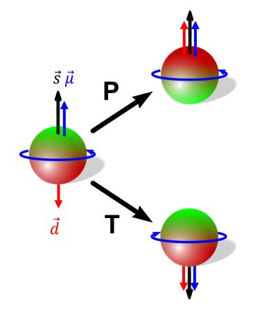
EDM measurements test violation of fundamental symmetries  $\mathcal{P}$ ,  $\mathcal{T}$  and  $\mathcal{CP}$  (via  $\mathcal{CPT}$ )
