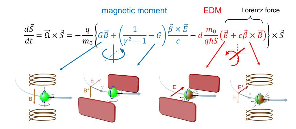
magnetic moment causes fast spin precession:  $\vec{s}_H \not\parallel \vec{p}$
