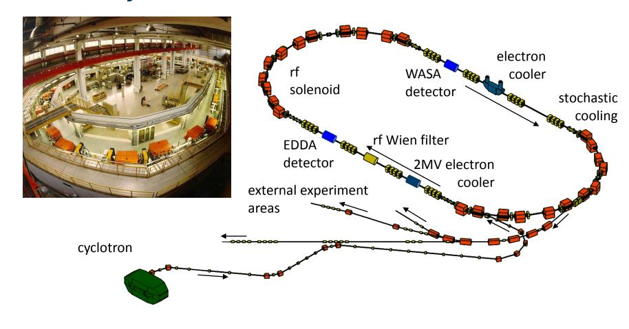
COSY provides cooled & polarized protons and deuterons with p = 0.3 - 3.7 GeV/c
