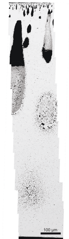
Figure C-2 - SEM panorama of polished cross-section from a phase inversion tape cast STF25 specimen.
