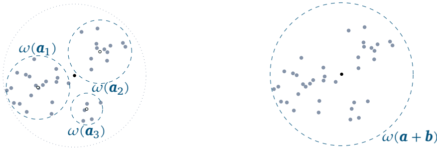
Figure 2.5: The multipole to multipole operator allows to shift multipoles around an old center to a new center.
