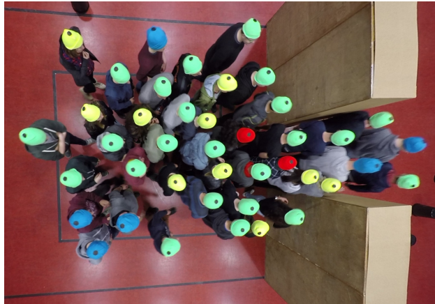
Fig. 4. Clogging in front of a bottleneck.
