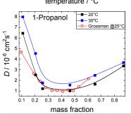
Around a mass fraction of 0.35 the diffusion coefficient shows a minimum. Only at very low concentrations single molecules diffusion is observed.
