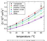
With increasing temperature diffusion increases, which is expected because the viscosity of solution decreases.
