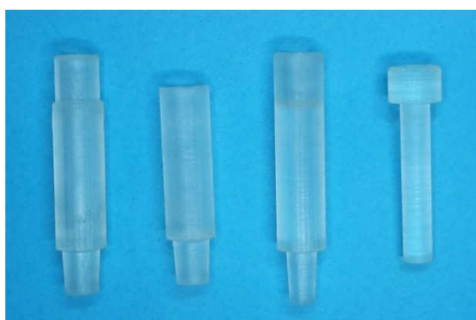
Figure 5. Picture of the 3D printed parts used in this research. Shown are from left to right: female Luer to filter holder adapter, filter holder, filter holder to male Luer adapter and the push rod for placing the filters inside the filter holders. The outer diameters of the filter holder as well as the adapters are 7.5 mm.
