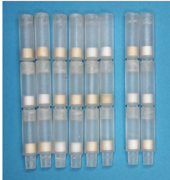
Figure 6. Picture of the stacked multi-filter columns. They are ordered in the same way as their measurement signals are shown in Figure 7. The left six columns (Column 1–6 in Figure 7) contain all possible combinations of 3 different coated filters, each flushed with both target antigens. The two columns on the right (A and B in Figure 7) are the ones where just one analyte was flushed over, they are stacked in the same order as column 1. All the filters are 5 mm high, and the outer diameters of the filter holder are 7.5 mm.
