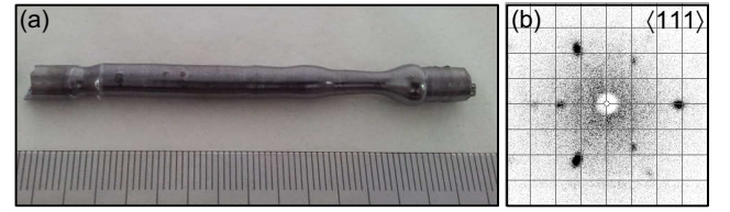
FIG. 2. Key characteristics of the single crystal grown for this study. (a) Optically float-zoned single crystal of \text{CuMnSb} . The scale on the bottom is given in millimeters. Growth direction was from right to left. (b) Threefold x-ray Laue pattern of a cubic \langle 111 \rangle axis.
