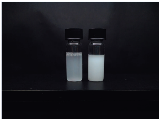
Fig. 4 Comparison between the homogeneously (MG 10 F) (left) and heterogeneously (MG 10 P) (right) crosslinked microgel particles in suspensions with c_{MG} = 0.5 wt%. The structural heterogeneity of MG 10 P is clearly visible as a difference between the turbidity of both samples due to stronger multiple light scattering in sample MG 10 P. 20
