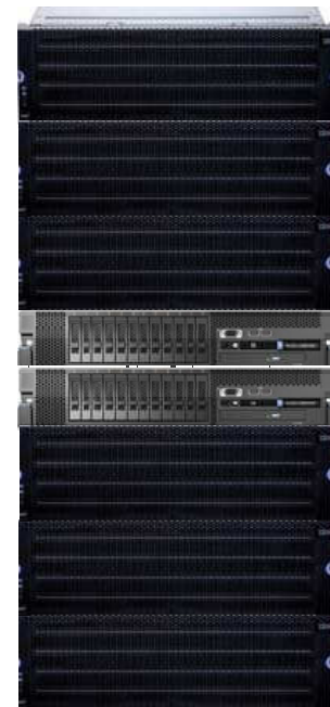
GSS 26: HPC Workhorse 2 x3650 servers + 6 JBOD Enclosures, 28U
