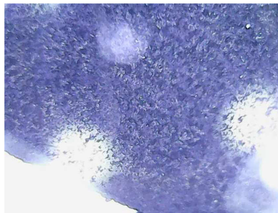
FIG. 20. Optical picture of the contact between a flat glass plate and a rectangular rubber block squeezed together in water. Note the granular structure which results from the rubber surface roughness. For the glass-rubber contact fully immersed in water, we cannot detect any time-dependent changes in the optical pictures. This is due to the rapid fluid squeeze-out and the fact that in the optical pictures the rubber-glass contact regions where the surfaces are separated by, say, 1 nm of water, look the same as when the rubber is in direct contact with the glass.
