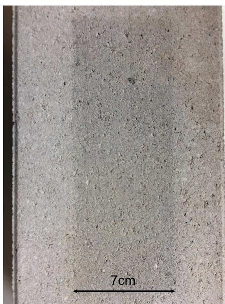
FIG. 21. The concrete surface used in the experiments. The dark region arose from transfer of rubber material (carbon black filled HNBR-50) to the concrete surface during sliding at v = 1 mm/s for two cycles (each cycle is 40 cm) at T = -40^\circ\text{C} .
