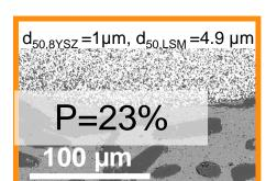
8YSZ/LSM=50/50%<sub>wt</sub> Co-sintered at <1300°C 5h d<sub>o</sub>: LA-950 V2 Retsch Horiba
