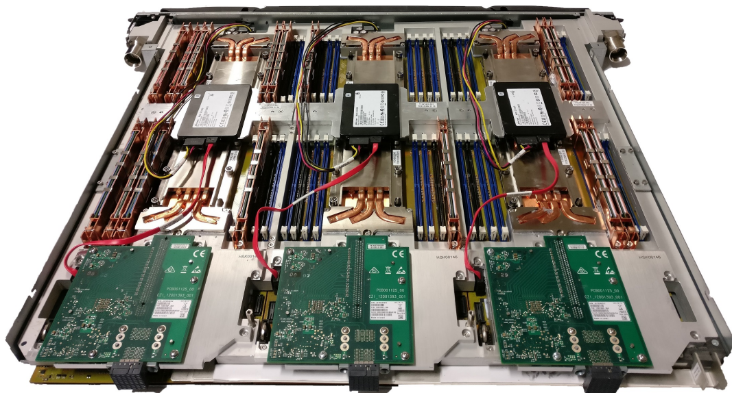
Figure 2: Example of a BullSequana compute blade encompassing three compute nodes. Please note that the shown local storage devices are not built into the JUWELS compute nodes. Copyright: Atos.
