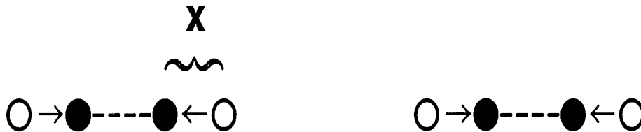
Figure 4.3: Definition of displacement x . The open circles denote the symmetric arrangement where intramolecular and intermolecular distances are equal. The length x is the displacement from the fully symmetric geometry.
